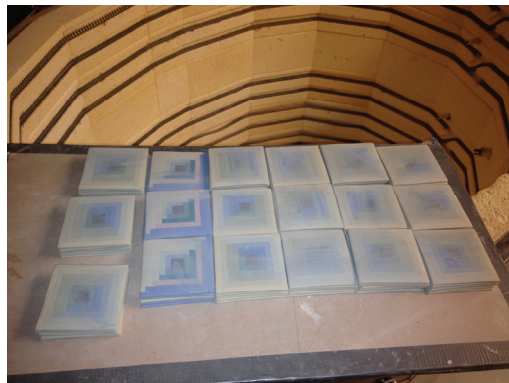
loading a kiln for bisque firing
